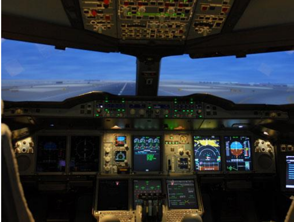
The cockpit has been designed to be similar to existing Airbus aircraft, thereby reducing the amount of training time needed for pilots.
